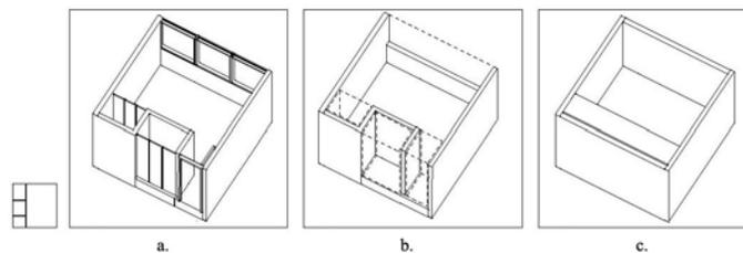
**Figure 4-1: Different levels of abstraction – a) architectonic, b) spatial, c) diagrammatic**
